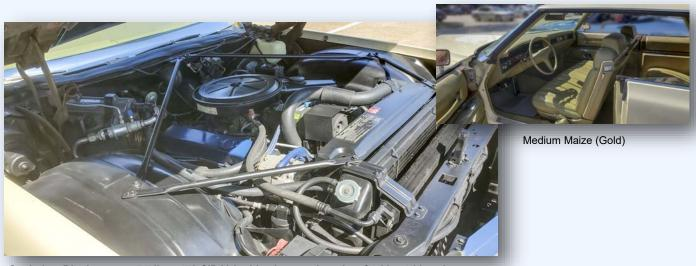
Statistics: Displacement:7.7 liter 472 CID V-8 with a bore and stroke of 4.30 x 4.06 and a compression ratio of 8.5 to 1, producing gross horsepower of 345 @ 4400 rpm and SAE net horsepower: 220 @ 4000 rpm. This engine usually had a Rochester Quadrajet 4MV carburetor. 0-60 mph in 10.1 sec, 0-100 km/h in 10.7 sec and quarter mile time is 17.5 secs.
