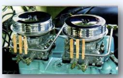
closer to the tank helps avoid "vapor lock" on older rides. My 1956 dual four barrel Eldorado Seville in Florida required repairing and replacing the in line fuel glass sediment bowl to restart. Cadillacs Cliff Wagner simply ran a fuel return line to the tank in 1956 and adopted by Cadillac nationwide.
